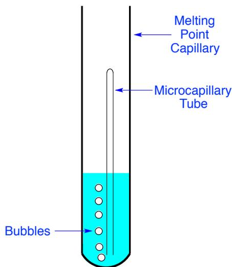
Figure 3. Micro Boiling Point Capillary
